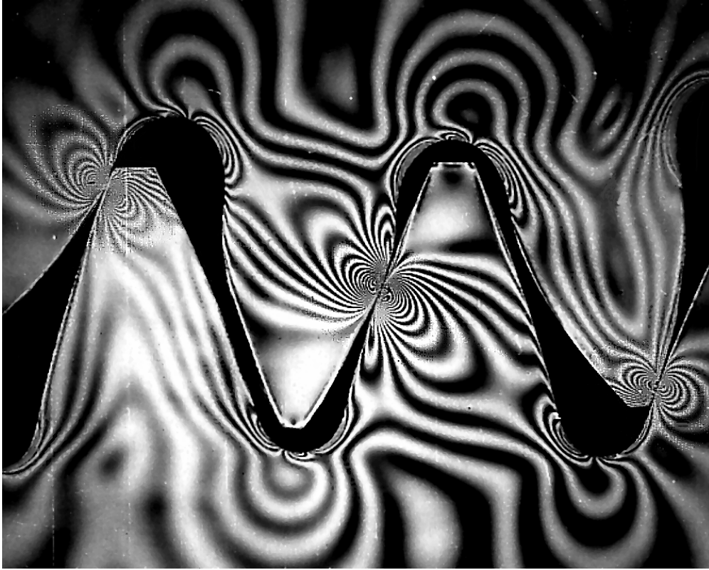
Figure 4. Photograph of the loaded HCR-gears photoelastic model in triple contact ( F_{bt} = 1913 N)
