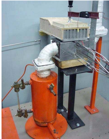
Figure 3 WHRS in a small steam generator with a single thermoelectric module (TEM)
