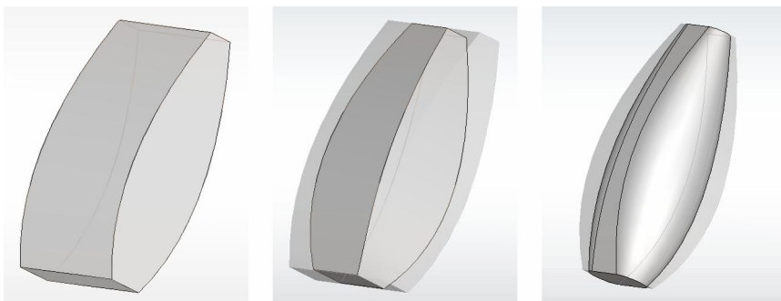
Figure 1. The initial stages: two profile cuts and two full-round radii are applied to a virtual block
