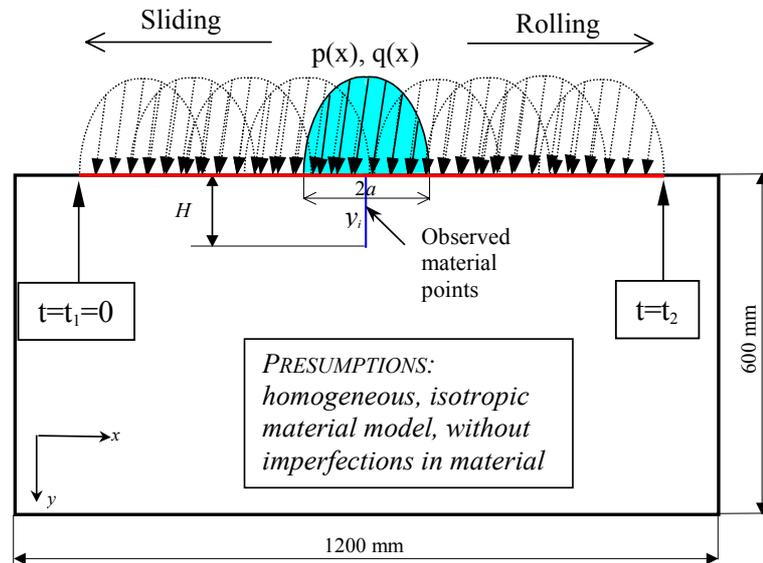
**Figure 1. General idea for determination of loading cycle at contact fatigue of mechanical elements**
