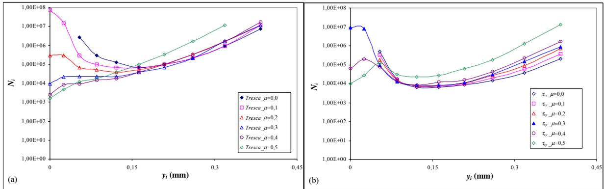
Figure 5. The number of loading cycles for fatigue crack initiation: (a) comparative Tresca based loading cycle; (b) shear stresses  $\tau_{xy}$  based loading cycle
