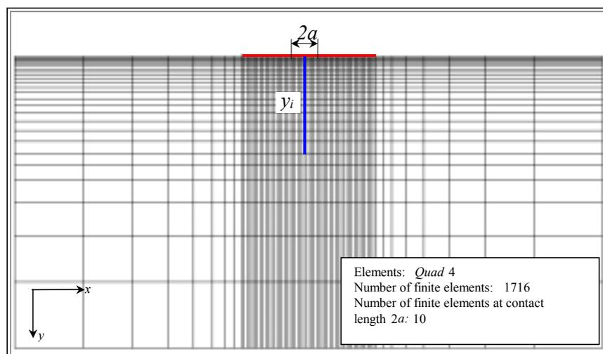
**Figure 2. Finite element model for determination of contact loading cycles**
