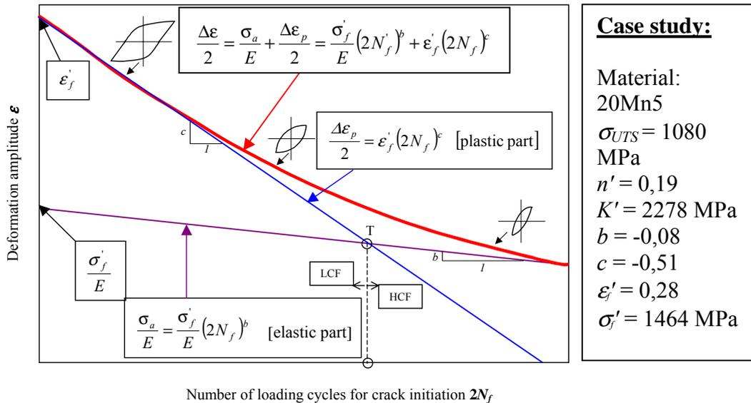
Figure 4. Strain-life ( $\epsilon$ - $N$ ) material curve and material properties [MSC/Corporation 1999]
