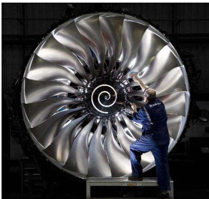
Figure 3a. Fan system [18] and Figure 3b. Fan blade showing fixings [19 p103]
