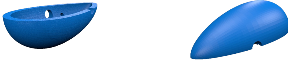
Figure 2. Half of a flute is reoriented so that support material is used only on the inside to preserve the outside surface finish of the artefact (Principle 2)
