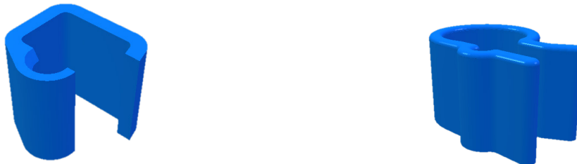
Figure 5. The profile of this clip is altered to provide a lower spring constant and be easier to use while the internal geometry remains the same (Principle 9)
