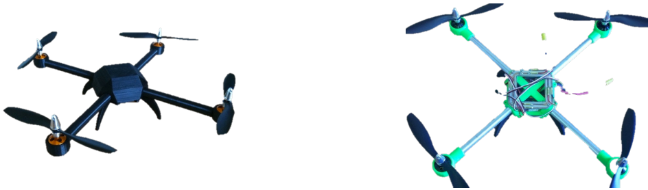
Figure 7. This quadcopter design is modified to use aluminum struts instead of being fully additively manufactured (Principle 22)
